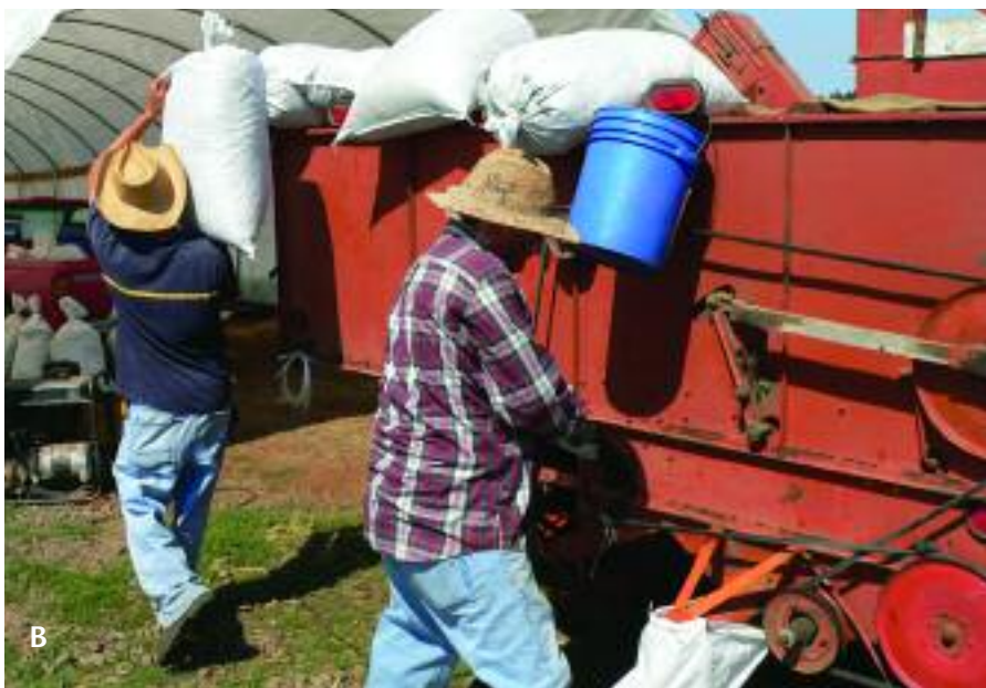
Figure 6. The plant material is placed on the belt feeder of the combine, then threshed and separated through screens (A). The seeds and small chaff are augured directly into seed bags (B).
