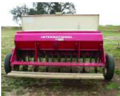
Figure 2. Our International seed drill with every other furrow opener removed.
