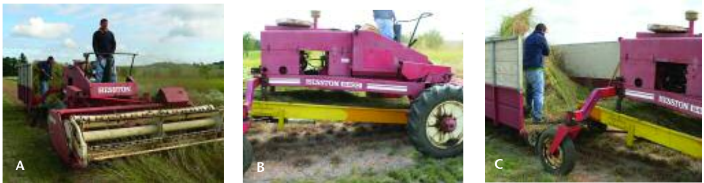
Figure 5. Bromus carinatus is cut with the swather blades (A). The material is conveyed (B) into a trailer pulled behind the swather (C). Photos by Lynda Boyer
